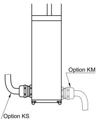
Mounting at lower end with bore hole Ø6.1 Option U6:
