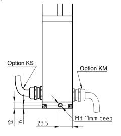
Mounting at lower end with bore hole Ø10.2 Option U10:
