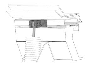
Fix the eyebolt in the coupling bracket using the bolt.
