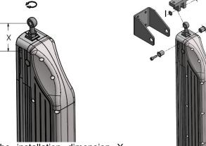
The installation dimension X can be set by moving the sliding blocks, fine adjustment takes place by turning the eyebolt.
