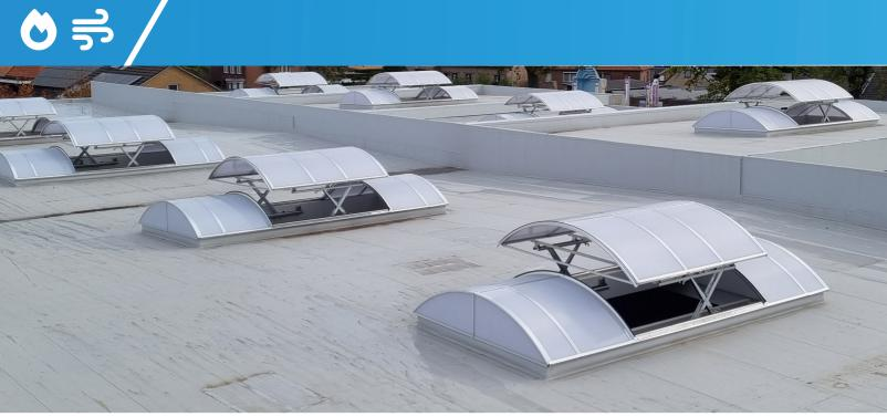
The mounting serves the purpose of opening and closing devices for natural smoke and heat evacuation such as skydomes and skylights. The scissor mounting is available in an electric version with electric actuators and in a pneumatic version with pneumatic cylinders.
