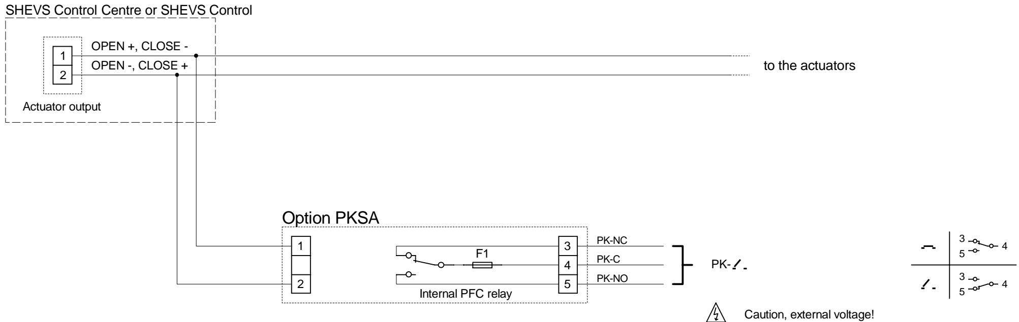
Contact load rating: 5A / 30V- / 230V~
